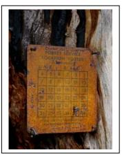
Land surveyors plotted out the west by dragging "40 chains" a mile long and marked a section. They would find the closest tree or rock to mark the section. Each section is 1 square mile and very noticeable when looking out of a plane flying over western states because roads and housing developments are developed within sections.
